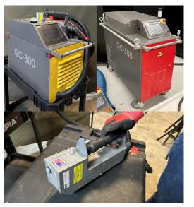
There is a multitude of laser lenses which changes how intense the beam is. The smaller the lens size, the smaller the surface area covered is but the more intense the laser is. The larger the lens size, the larger the surface area covered is, but the weaker the laser is.
