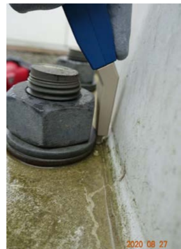
Photo 2. Long angled pencil probe gaining access to welds behind bolted flanges.
