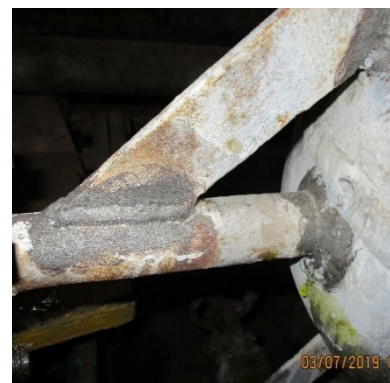
Spot area of bore weld after Laser Cleaning
